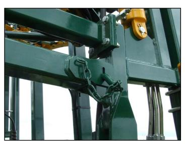
Pin Locked in Transport Position
